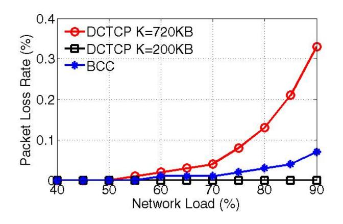
BCC keeps low packet loss rate
