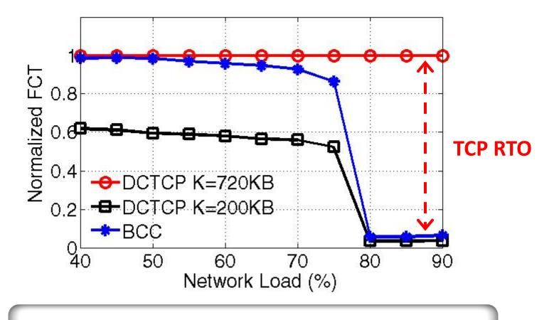
BCC keeps low packet loss rate
